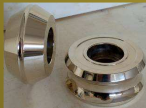
Pipe mandrels and rolls
