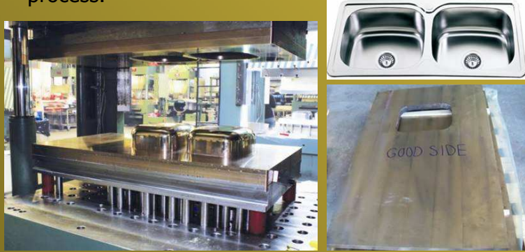
Deep drawing process for the production of stainless steel kitchen sink by "deep drawing dies"
