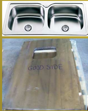
Deep drawing process for the production of stainless steel kitchen sink by "deep drawing dies"
