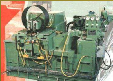
Flash welding process of wheel rim and electrodes
