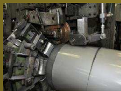
Seam welding of barrel by discs
