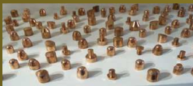
Spot welding electrodes and process
